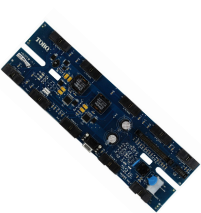
R102-3497-4.0 Timing Mechanism - Version 4.0 (comes with current firmware)
