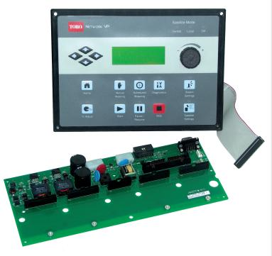
Upgrade Kit – Network LTC® Plus to Network VP® Upgrade kits include a faceplate, power distribution board, and interface cable. Full installation can be completed in minutes per controller.
