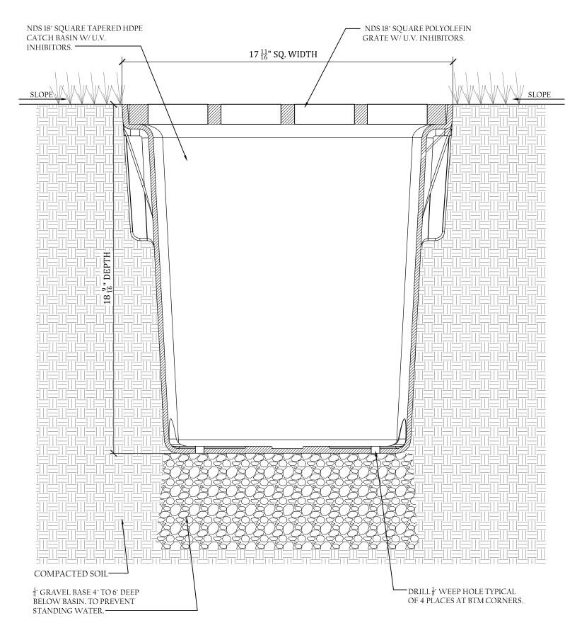
GRATE TO BE ATTACHED TO CATCH BASIN WITH SCREW PROVIDED AT TIME OF INSTALLATION.
