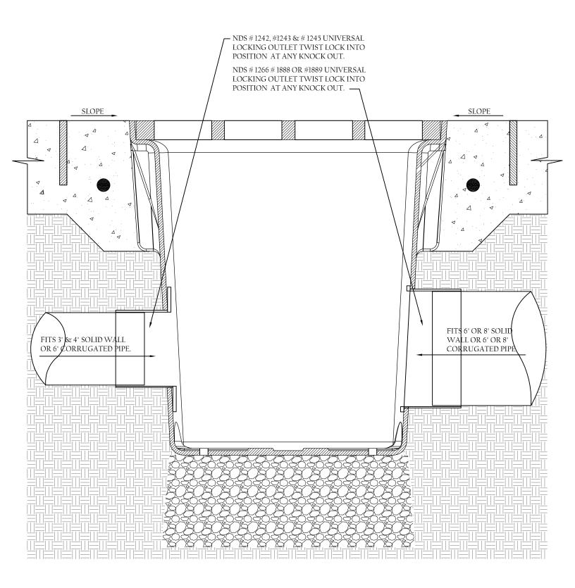
• NDS ADAPTERS THAT FIT THIS BASIN ARE AS FOLLOWS. #1242, #1243, #1245 #1266 #1888 & #1889 USE #1206 IF PLUGGING AN OUTLET. INCLUDES (2) #1890 REDUCER RINGS USED WITH SMALLER CONNECTIONS.
