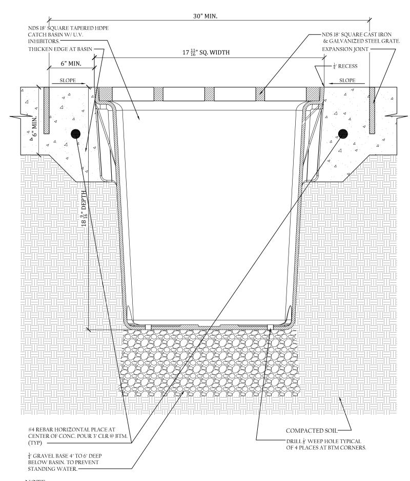
GRATE TO BE ATTACHED TO CATCH BASIN WITH SCREW PROVIDED AT TIME OF INSTALLATION.
