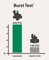
If high water pressure strikes, you need to be prepared for the worst-case scenario. For the Burst Test, we ramped up the pressure as high as it could go. We did the same for the valves of a leading competitor. The results were telling. While the competition exhibited body-to-bonnet leaks under pressures as low as 100 psi (6.9 bar), the PGA valve held strong, even at 440 psi (30 bar).
