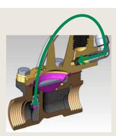
Filtered water flows directly through the contamination-proof bypass tube.
