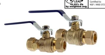
Standard compression valves can be used to make connections between Copper, Brass, Aluminum, Plastic, CPVC & Pex tubing. Not recommended for use with steel tubing. They are designed for use with tube manufactured to CTS-OD copper tubing sizes (outside diameter controlled). NOTE: A brass insert must be inserted into Soft Copper, Aluminum, Plastic, CPVC & Pex tubing to put 360° of even pressure on the tubing, to make a round rigid profile that will ensure a tight seal.
