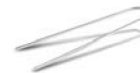
TLS6 6" Soil Staple (Place approximately every 3' of tubing, plus two on each tee, elbow or cross.)
