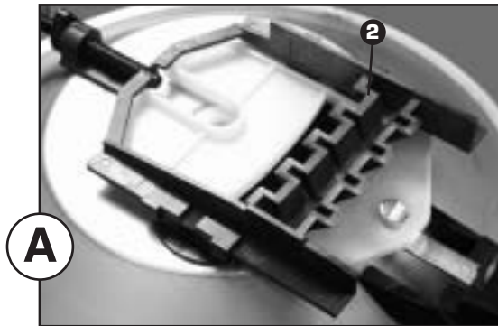
Note the relationship of the rate gate opening to the front side of the ramp.
